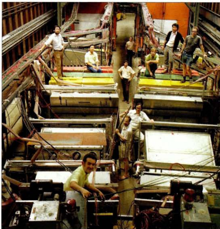
The muon pair spectrometer which discovered the \psi(3700) resonances at Fermilab in 1977. (Fermilab Visual Media Services.)
