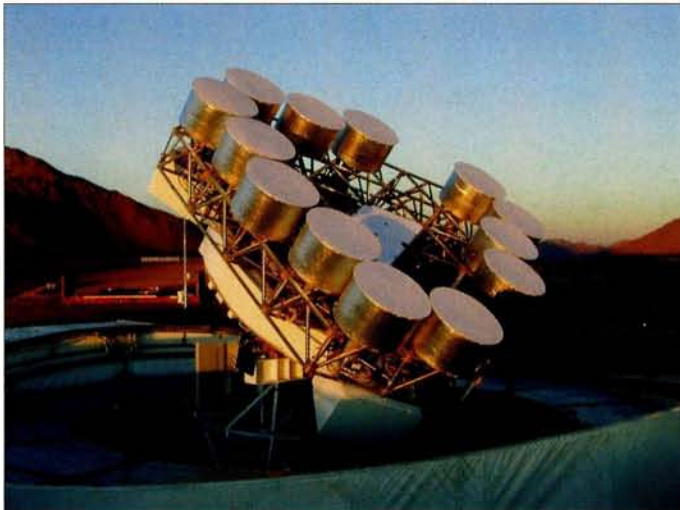
Left: CBI's 13 radio antennas. Right: the CBI power spectrum (with error bars in blue and green) compared with results from other experiments. (CBI/Caltech/NSF.)
